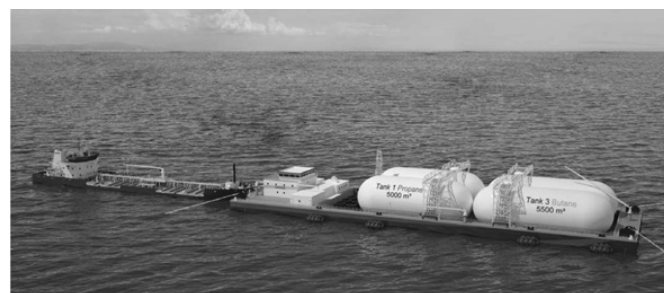
Figure 4: Small-Scale LPG FSU (Floating Storage Unit)
